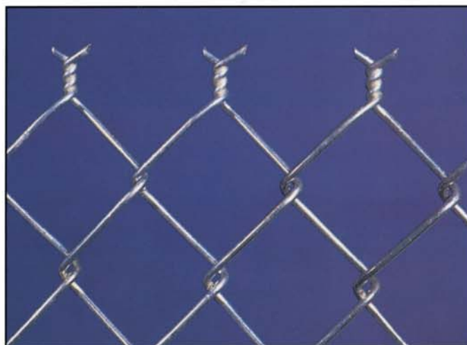
Right: GAW fabric. The GAW process guarantees that cut ends will be coated with the same quality material and protection as the rest of the fabric. The pre-coated process provides no such guarantee.
