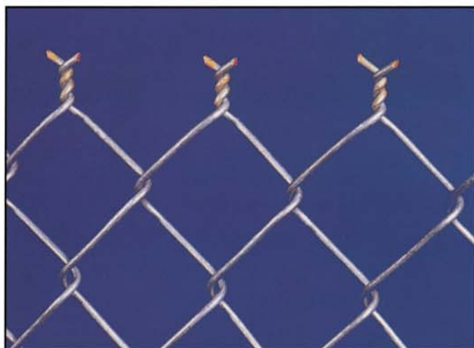
Left: Precoated fabric with uncoated tips. With pre-coated fabric some manufacturers coat the bare cut-ends, but many don't. No one coats the ends with the same material that protects the rest of the fabric.
