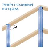
**NOTE:** If the ground slopes, be sure to cut both rail-ends diagonally to allow a flush fit against the post.
