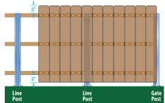
Typically pickets are positioned 2" above ground level and extend 8" above the top of the top rail.
