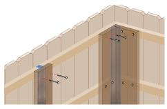
Finish the installation by adding 1x6 cover boards over the PostMaster PLUS posts.
